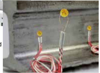
Railway axle load measurement
