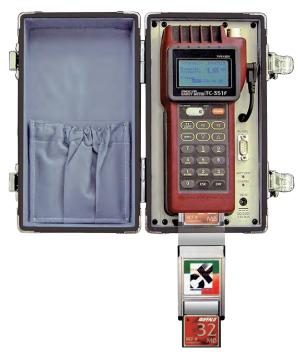
The indicator indicates results of analyses and also saves them into CF card. Measurement/Analysis software (TC-7100) is required for measurement system with personal computer. In this system, data indicated on the indicator are transferred to the computer through the indicator without modification. Personal computer displays waveforms of load and displacement and also processes each analysis.
